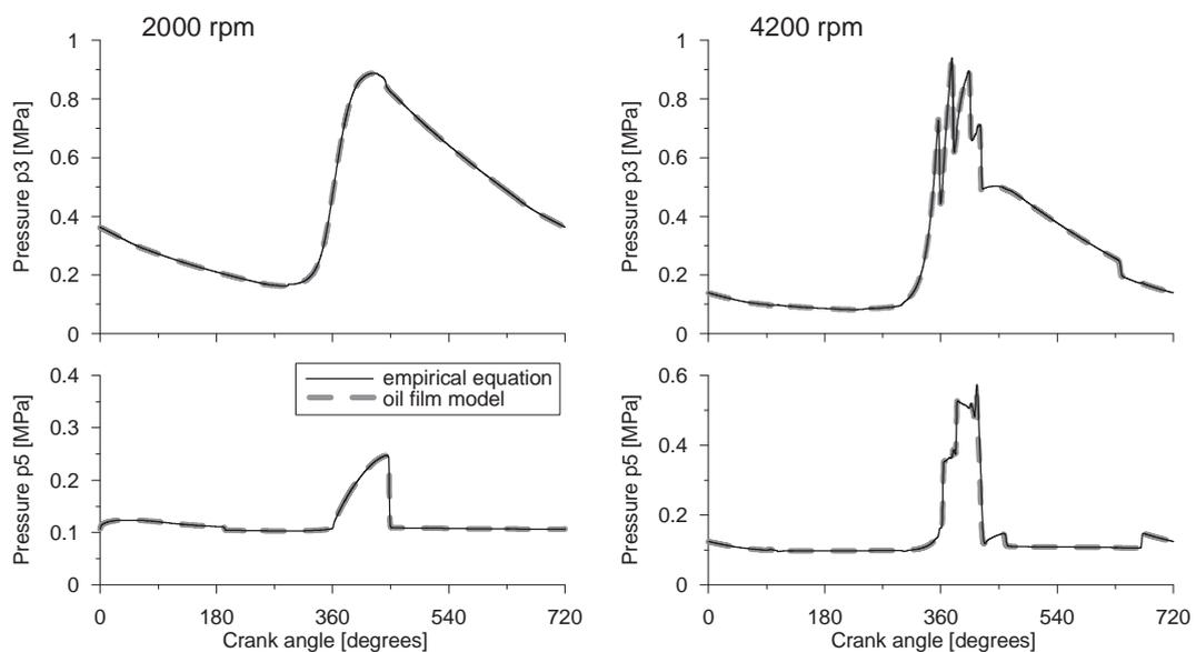
Fig. 6. Pressure courses in the inter-ring spaces calculated for friction forces calculated using empirical equation and oil film model for the engine full load at 2000 rpm (left) and at 4200 rpm (right)
