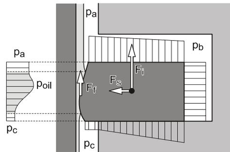
Fig. 2. Assumed pressure distribution and forces acting on the ring
