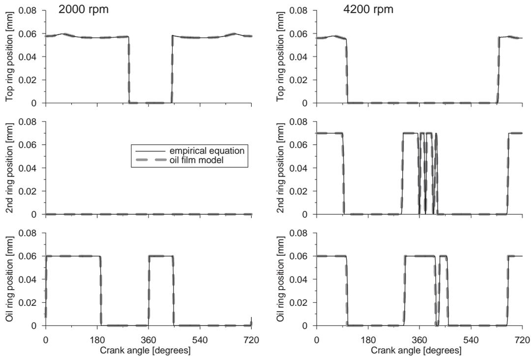
Fig. 5. Axial displacements of rings in the piston grooves for friction forces calculated using empirical equation and oil film model for the engine full load at 2000 rpm (left) and at 4200 rpm (right)
