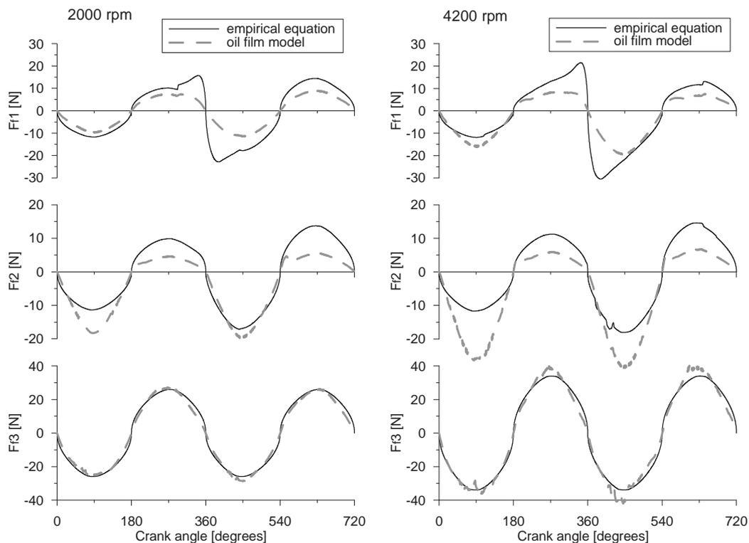
Fig. 4. Friction forces acting on top ( $F_{f1}$ ), second ( $F_{f2}$ ) and oil ring ( $F_{f3}$ ) as function of crank angle calculated using empirical equation and oil film model for the engine full load at 2000 rpm (left) and at 4200 rpm (right)
