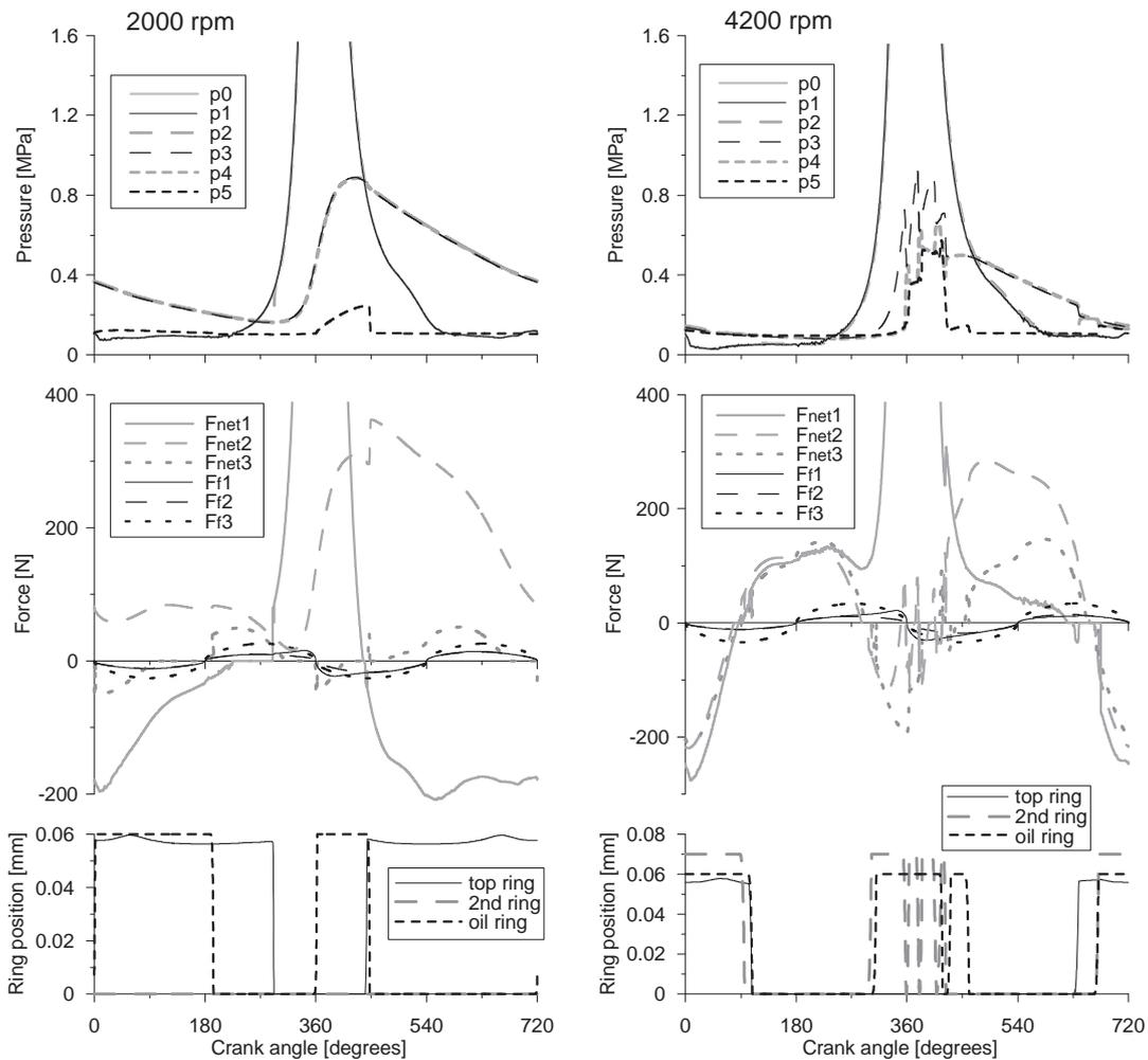
Fig. 3. Pressures in inter-ring spaces, friction and net forces acting on rings and axial positions of rings in piston grooves determined for engine full load at 2000 rpm (left) and at 4200 rpm (right)
