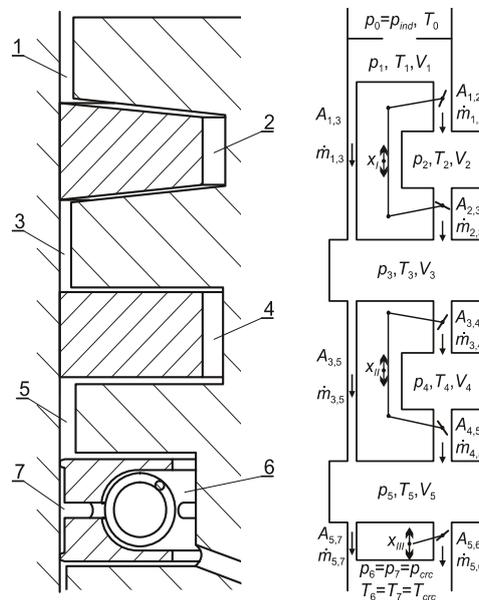
Fig. 1. Schema of the ring pack and corresponding model of labyrinth seal
